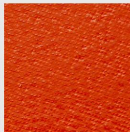
COATED SILICA CLOTH Temperature Tolerance 1,800 °F Continuous
