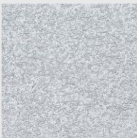
KEVLAR Resistant to chemicals and acids; heat resistant up to 600 °F
