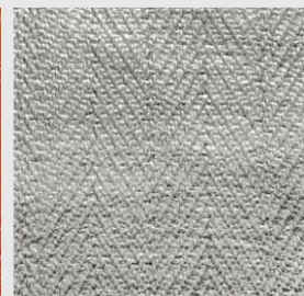
ALUMINIZED KEVLAR Resistant to heat and abrasions; heat resistant up to 600 °F
